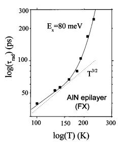
FIG. 5. Temperature dependence of the radiative decay lifetime of free excitons in AlN. The solid line is the fit based on a theory of free exciton dissociation in Ref. 15.
