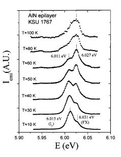
FIG. 2. PL spectra measured at different temperatures for an AlN epilayer. The arrows indicate the PL spectral peak positions of the bound exciton  $(I_2)$  and free exciton (FX) transition lines.
