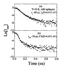
FIG. 3. Temporal responses of PL emissions measured at 10 K at the bound to perform exciton and free exciton spectral peak positions in an AlN epilayer.
