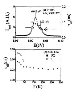
FIG. 4. (a) Emission energy dependence of the decay lifetime of the bound exciton and free exciton transition lines in an AlN epilayer measured at 10 K. The time-integrated emission spectrum is also included. (b) Temperature dependence of the recombination lifetime of the bound and free excitons measured at their respective spectral peak positions.
